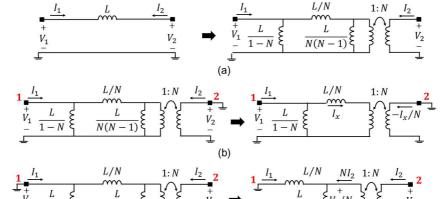
Fig. 2. (a) Norton transformation of a series floating inductor; (b) equivalent circuit for  $y_{11B} = I_1/V_1$  and  $y_{21B} = I_2/V_1$ ; (c) equivalent circuit for  $y_{12B} = I_1/V_2$  and  $y_{22B} = I_2/V_2$ .
