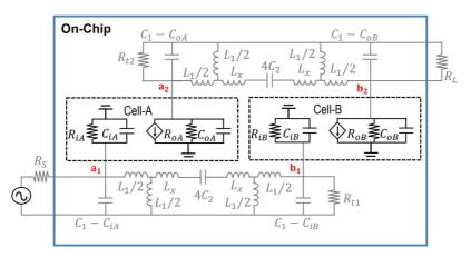
Fig. 4. Circuit diagram of the band-pass DA with representation of the input and output impedances associated with each gain-cell.
