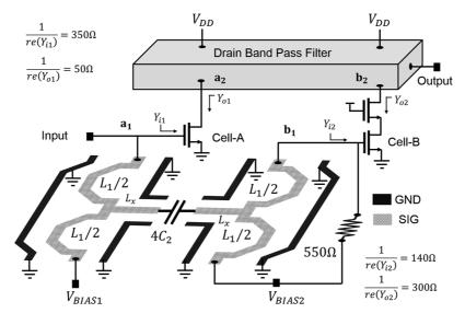
Fig. 5. Circuit diagram of the BPDA.
