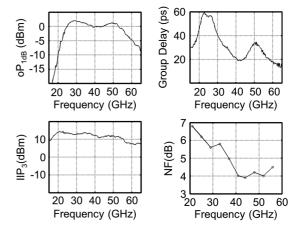
Fig. 9. Compression-point, group-delay, and IIP3 characterization versus frequency.
