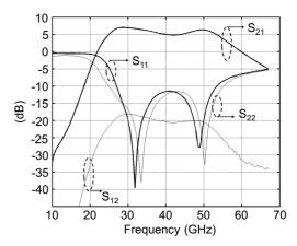
Fig. 7. BPDA measured S-parameters.
