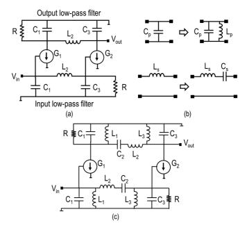
Fig. 1. (a) Canonical form of the LPDA (b) low-pass to band-pass filter transformation (c) canonical form of the BPDA.
