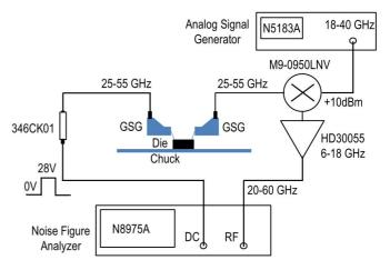
Fig. 8. Setup for BPDA noise characterization using the N8975A noise-figure analyzer.
