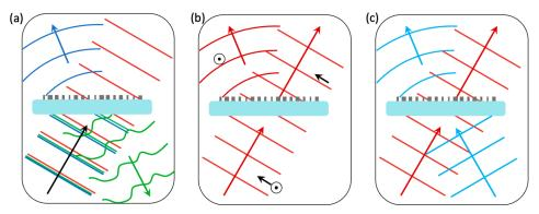
Figure 4. (a) Schematic of wavelength multiplexing where the metasurface imposes different transformations for different wavelengths (colors). (b) Polarization multiplexing where the transformation is different depending on the polarization. (c) Angular multiplexing where wavefronts incident at different angles experience very different transformations.
