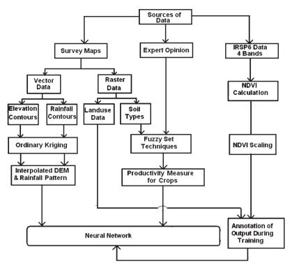
Figure 2. Schematic diagram of the methodology.
